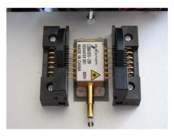
butterfly-package laserdiodes (specify pinout)
